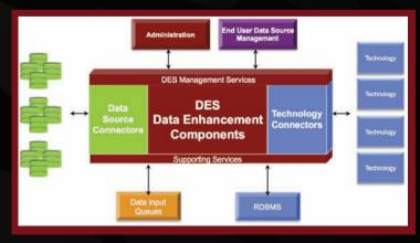
DES now processes the information record in its data base, communicates with the Data Source and causes the necessary updates to happen to the content stored in the Data Source.
